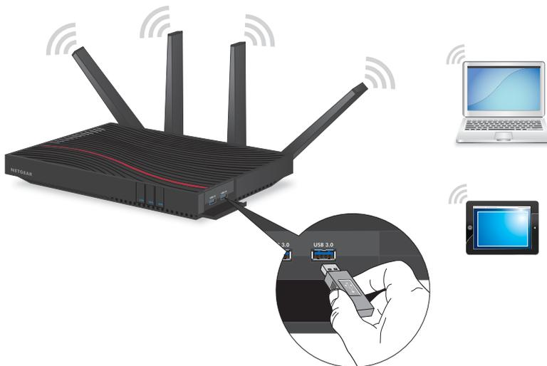
2. If your USB storage device uses a power supply, connect it.
